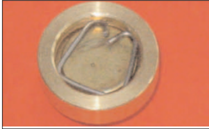
4.3: “Fit the recovered retainer spring clip, making sure its two spring ‘ears’ are uppermost, away from the disc.”.
