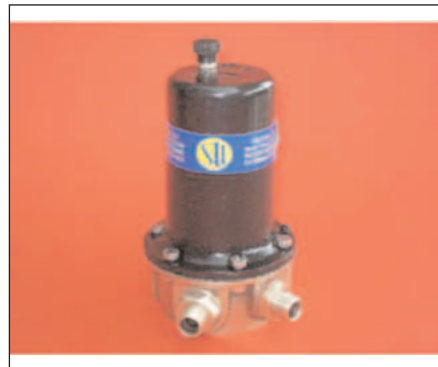
A refurbished SU pump
